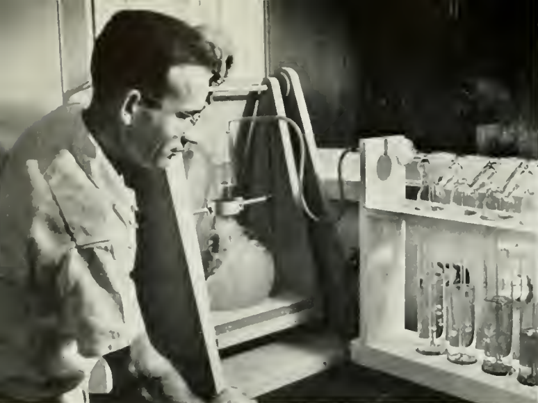
E. J. WOOD, RESEARCH CHEMIST, MANIPULATES A BUBBLING GAS TO PURIFY A SOLUTION WHICH IS BEING ELECTRICALLY HEATED AND SHAKEN IN THE PYREX FLASK.
