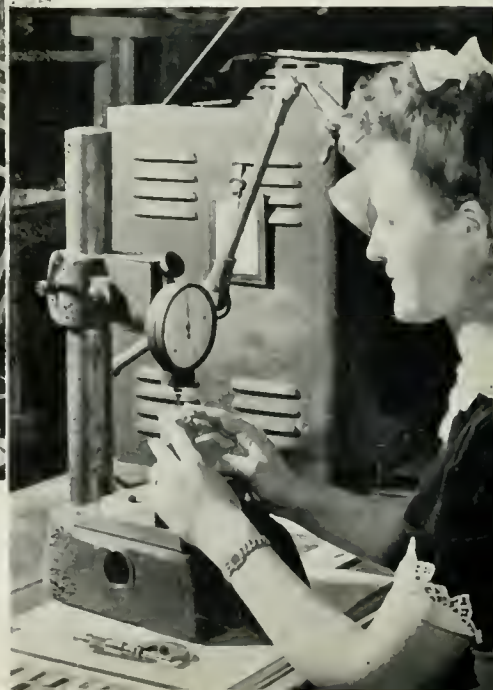
ANNA MAY GALLAGHER, RCA VICTOR WAR WORKER, GAUGES THE THICKNESS OF CRYSTAL BLANKS.
